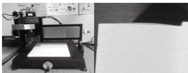
(a) Machine tool (Kitmill RD 300) (b) Machining result Figure 5 Machine tool and Machining result
