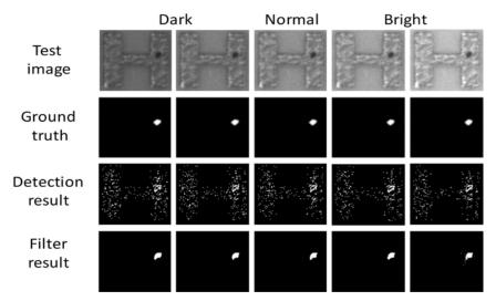
Fig.2 some example of inspection results under different illumination conditions.
