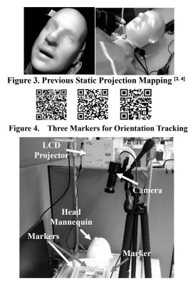
Figure 5. Dynamic Projection Mapping System Configuration
